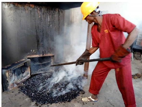
Figure 43. Unloading of charcoal from the oven. Agrovalor RCI Project (Nitidæ, 2017-2021).
