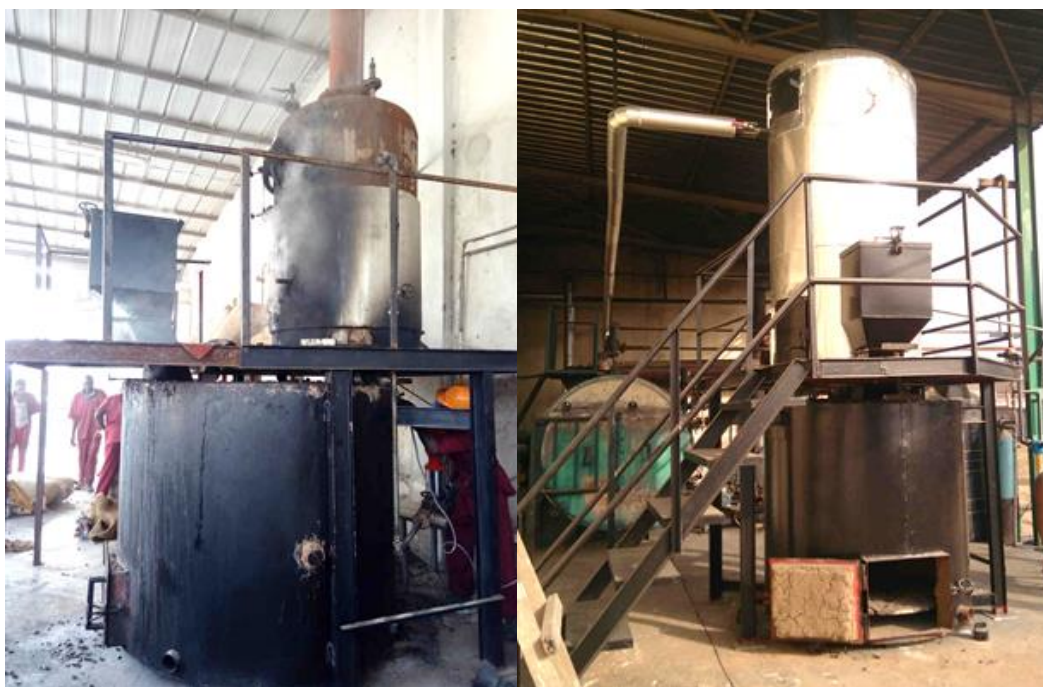
Figure 40. Two pyrolysis furnaces in West African factories, with the boilers above.
