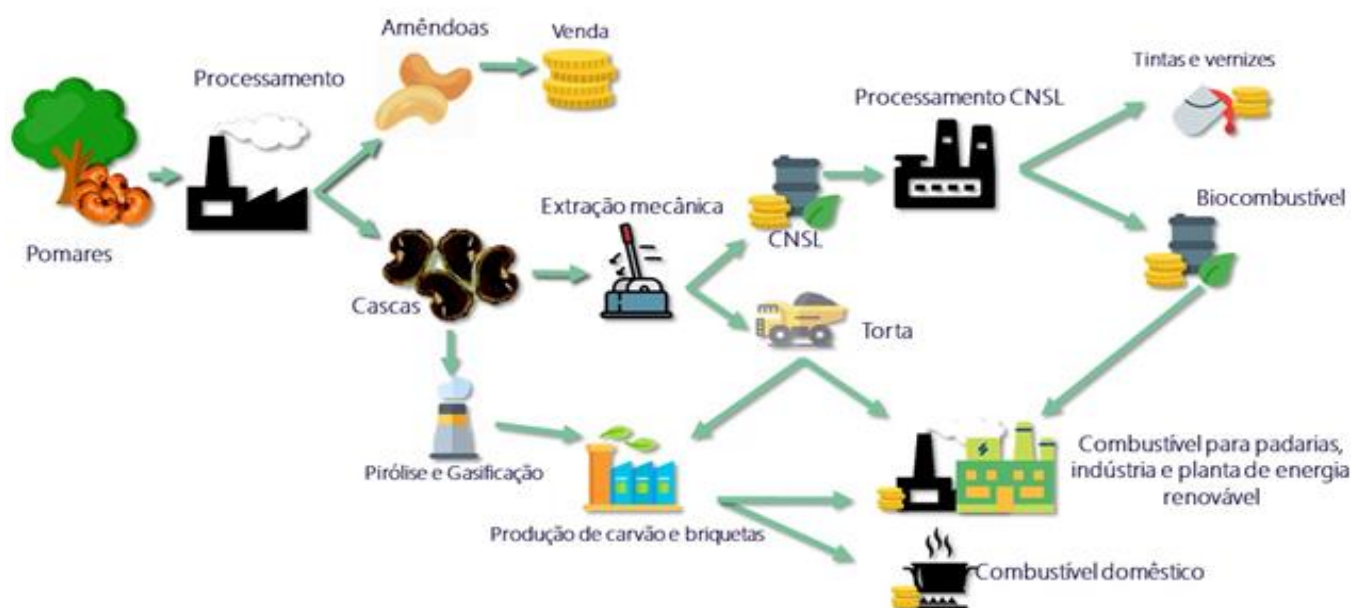
Figure 27. Optimized chain of cashew nut by-products valorization in Mozambique.
