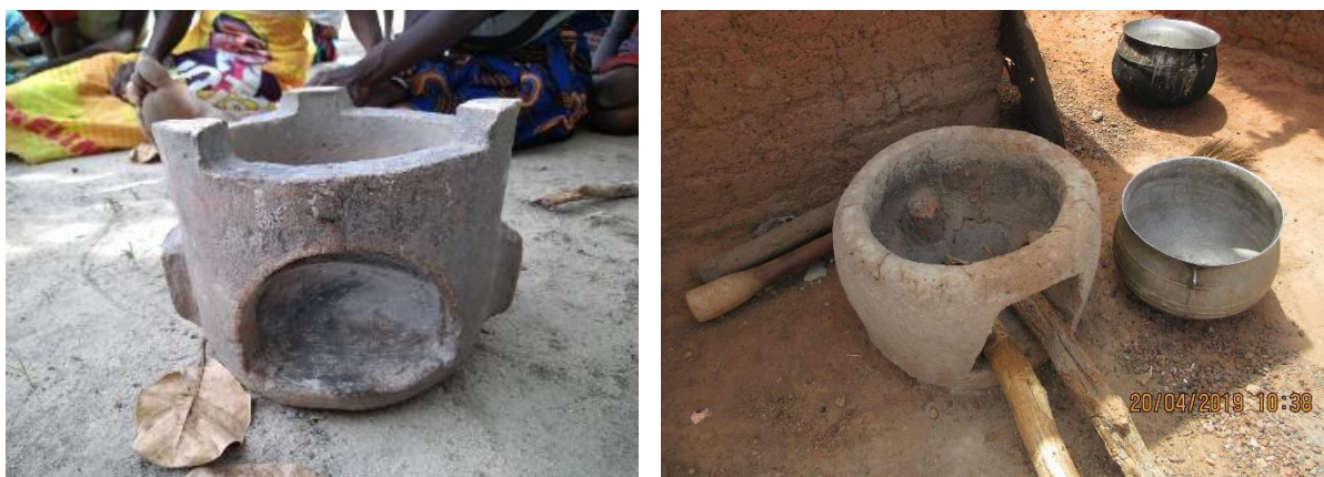
Figure 20 : Improved cookstoves in clay. Left: model spread by COSV some time ago around the BZ communities; right: locally hand-made improved cookstove from Burkina Faso)
