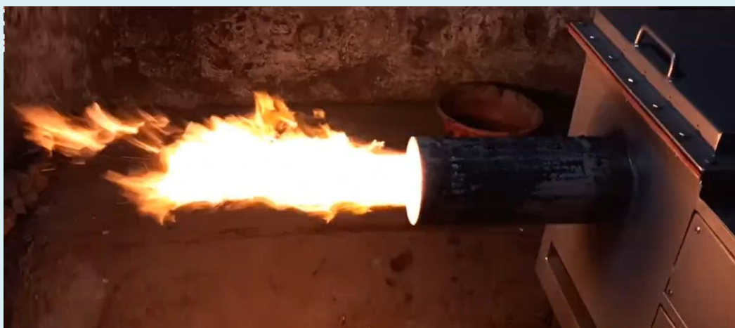
Figure 15. Solid biomass burner adapted to cashew shell cake for a proper combustion at a small scale.
