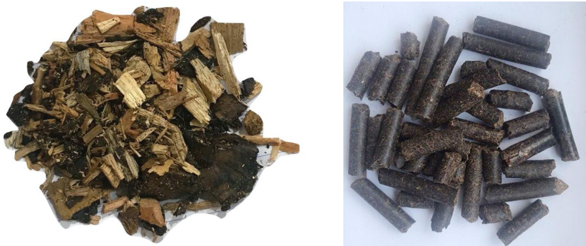
Figure 17. Cashew shell cake sold mixed with other waste biomass (left), and shell cake pellets (right)
