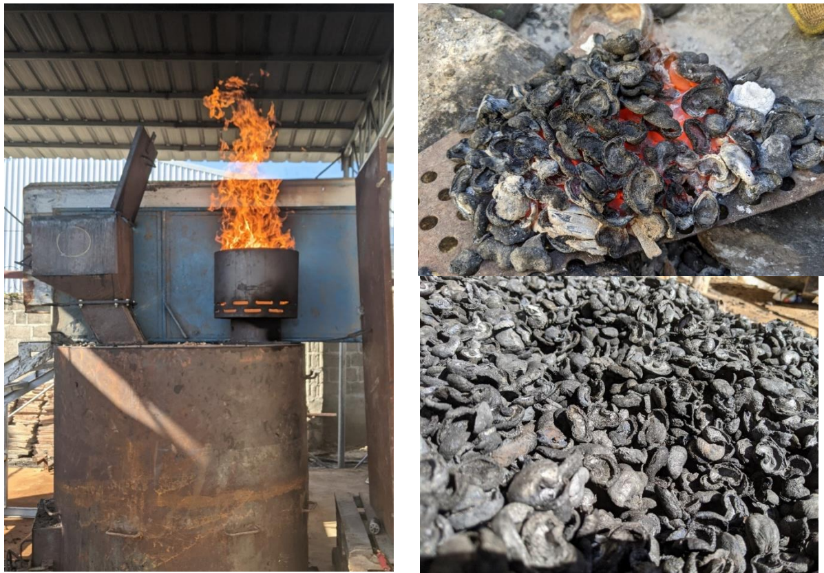
Figure 25. Flammable pyrolysis gas is produced at the burner of the H2CP. At the end of the operation, shell charcoal is obtained
