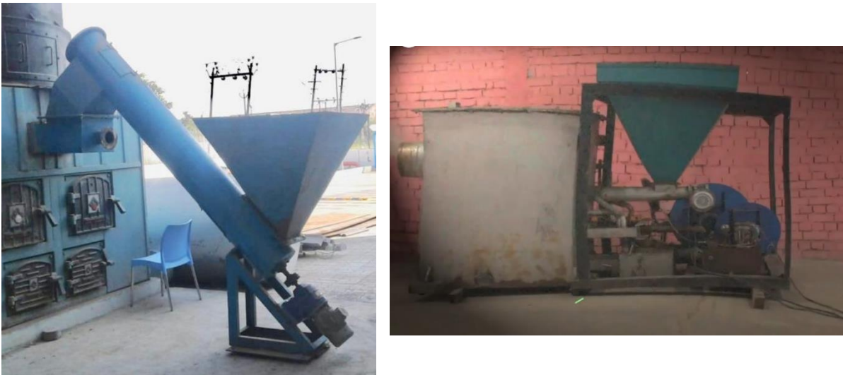
Figure 18. Auto feeders with conveyor (left) and biomass burners (right) are the most extended technologies to cleanly burn waste biomass, as they require minimum changes in the existing heating device (boiler or kiln).
