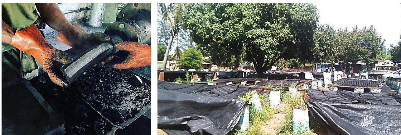
Figure 31. Verde Africa's charcoal briquettes obtained in an extruder (left), then dried in racks
