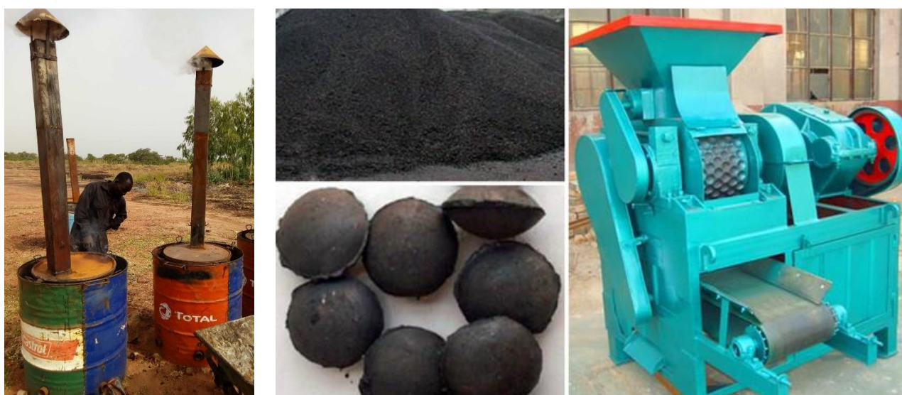
Figure 32. A barrel kiln is employed for the carbonization of coconut shells (left). The milled charcoal is then compacted in a briquetting machine (right).
