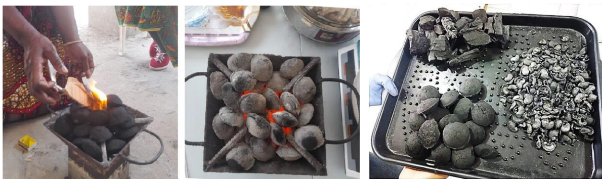
Figure 28. Cooking tests using cashew shell briquettes (left and middle); the three materials tested by the BECT laboratory for comparative combustion performance and emissions testing (right).
