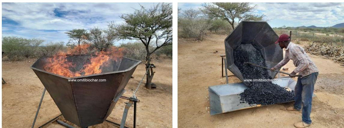
Figure 6 : Photos of Kon Tiki kilns in Namibia (Source: Omiti Biochar)
